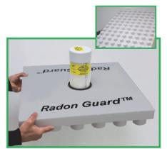
**Radon Guard®** insulation is patented sub-slab depressurization panel. The interconnected channels on the underside of the panel direct soil gas movement between the ground and the air barrier system to a vent pipe in slab on ground applications as required by National Building Code of Canada 2010, Section 9.13.4. The vent pipe is required to connect to a radon gas mitigation system as per applicable code.
